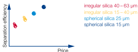
Comparison of separation efficiency and price of irregular versus spherical silica
